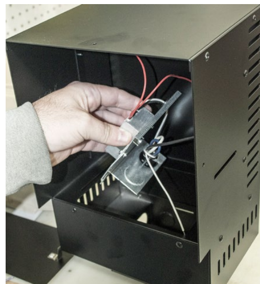
Step 5- After assembly has been removed, replace with new transformer. Reverse steps to re-install.
