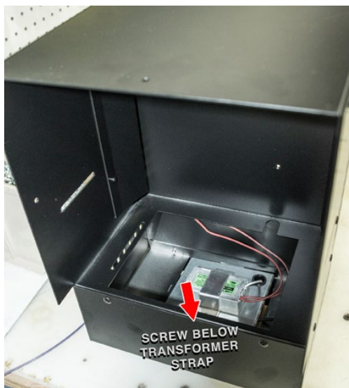
Step 4- Remove transformer assembly by removing 1 screw. Screw located below transformer strap.
