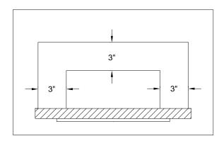
DO NOT INSTALL INSULATION WITHIN 3" (76mm) OF FIXTURE SIDES OR WIRING COMPARTMENT
