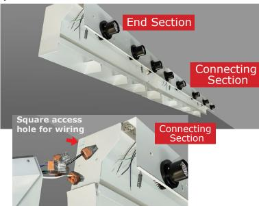
**Step 4**- Connect wiring of newly installed section with existing section. Position and clip new section into existing section. Make sure to use mounting screws to secure each section to ceiling
