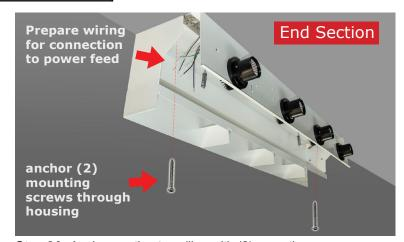
**Step 2A**- Anchor section to ceiling with (2) mounting screws. **DO NOT** forget to use proper support above ceiling to anchor mounting screws and sections into ceiling.
