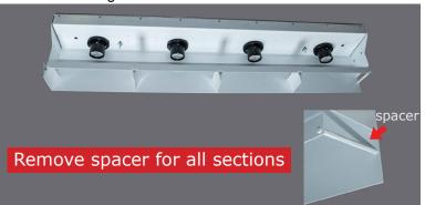
**Step 3-** Remove screw holding spacer. If spacer is not removed, section will not clip into existing section in ceiling. Repeat this step when installing new section.
