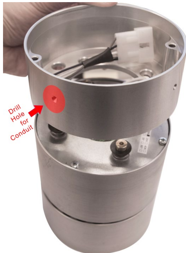
Step 2- Cut-out 3/4" hole centered around punchout holes in surface junction box (up to 4 holes)
